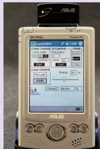
PDA software interface for controlling laser operation
