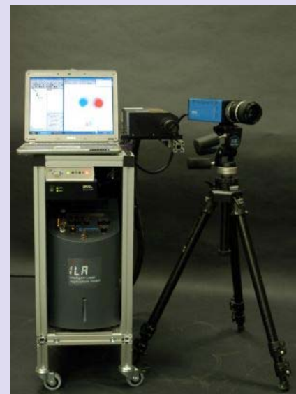
Standard 2D PIV System in Notebook Configuration. Includes pco.1600 PIV Camera, connected via Firewire link
