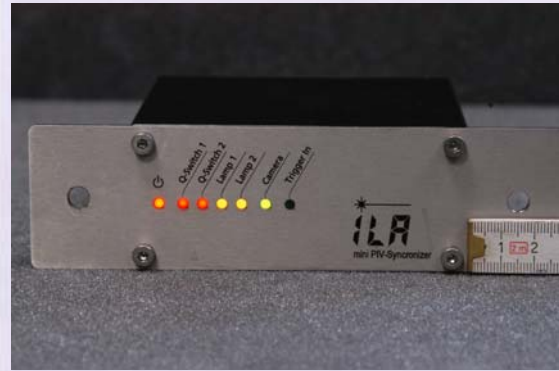
MiniPIV-Synchronizer front panel with status LEDs
