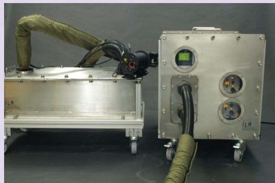
Meet CARLA, a temperature and pressure controlled laser light sheet delivery system, specially designed for CIRA's icing wind tunnel
