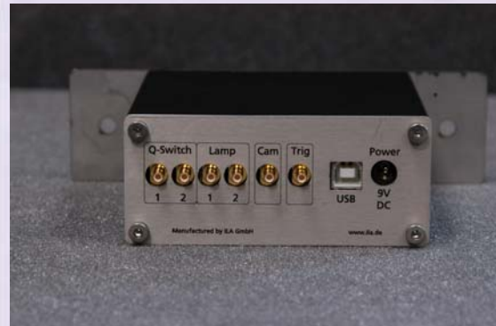
Back panel with I/O and power sockets and USB port
