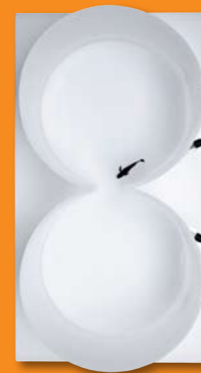
Shuttle Box for preference temperature studies
