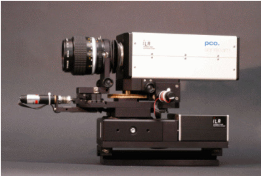
Complete motorised camera unit, with rotation, tilt and focus control
